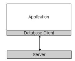
The figure above shows an application with the database-programming interface, which is connected to the database server.
